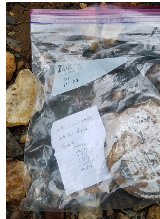
Labeling a bag with a time-stamp can allow for collation with GPS tracking information. A photo of the bag in situ allows for further contextualization.
